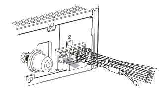
• The pin arrangement for the ISO connectors depends on the type of vehicle you drive. Make sure to make the proper connections to prevent damage to the unit.
